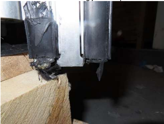
Picture 17 Internal and external rebate seal, casement at bottom
